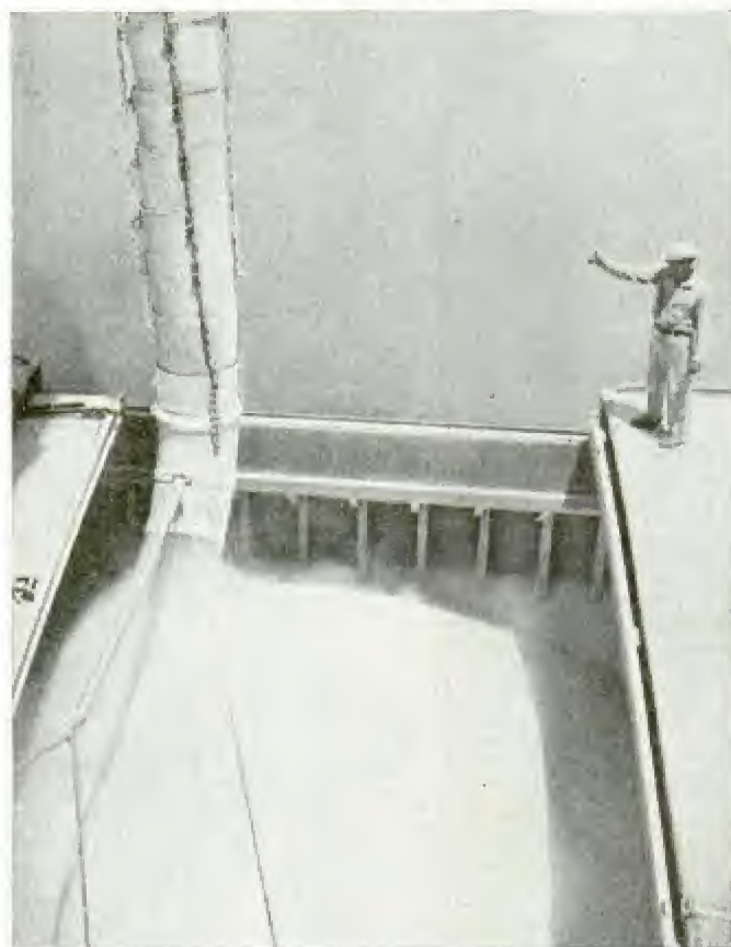
Drilling a hole for a charge of explosive that will break up the storage pile so it can be loaded in cars by huge shovels. Below, a golden stream of sulphur dust flows through spout from weigh house to load a Mississippi River barge in Louisiana
